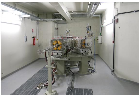
Photo showing the two sub-branches of the Trento proton irradiation facility, namely the 0° line (left) and 30° line (right)
