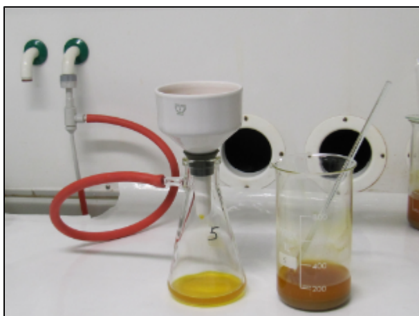
Figure 1. filtering the digested sample using Bühner-funnel and suction
