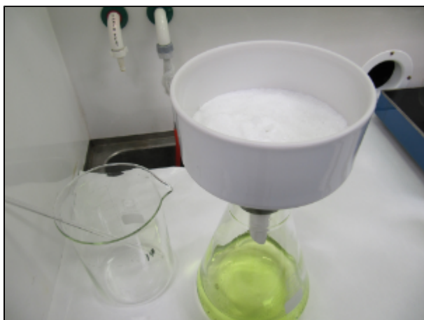
Figure 2. Filtering the oxalate precipitation using Bühner-funnel and suction
