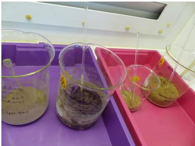
17. When a constant weight has been reached, tare a counting container, and transfer the standard into it, ensuring that the material reaches the top on the container. Take extreme care not to lose any material during the transfer (ensure work is performed in a foil tray).
