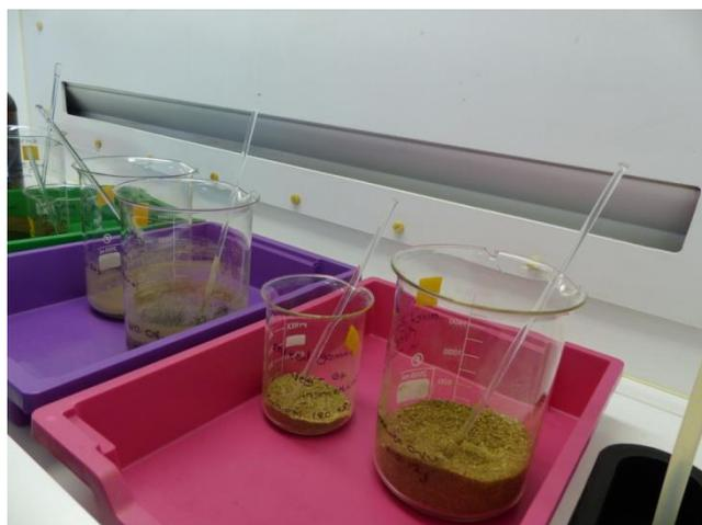
14. Depending upon the geometry of the container diluted reference solution is added to approximately 100 or 700 ml of methanol (volume dependent upon amount of calibration material).
