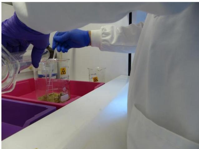
15. Methanol is added with gentle mixing to the reference material with gentle mixing, ensuring no losses. Add more methanol if required to the mixture and mix, repeat mixing every few hours to avoid the calibration material 'caking' and sticking to the sides of the beaker. Allow the standard to dry slowly to a constant weight.
